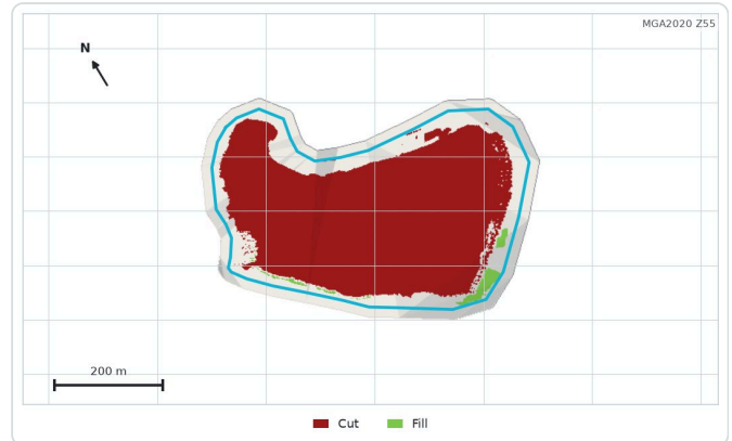
Stockpile (OBJ). Net -1,546,769 m 3 .
